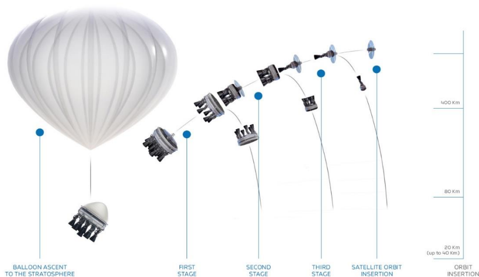
Figure 3: Flight cycle of Bloostar [9]
